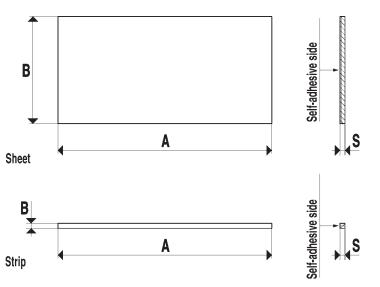
The same kind of foam rubber used for making suction cups can be supplied in sheets or strips, with the sizes shown in the table.
