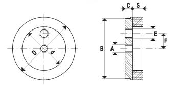
These cups are the same foam rubber cups as previously described, fixed on a proper support in anodized aluminium.
